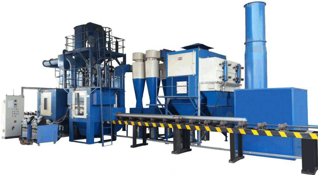
INLINE PIPE BLASTING & COATING MACHINE
