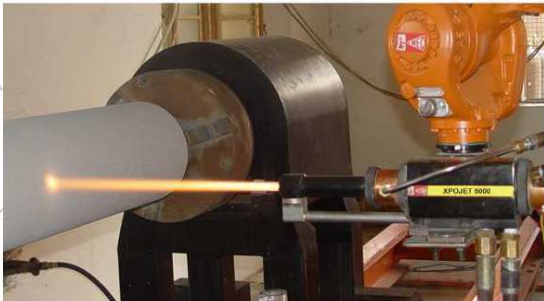
XPOJET LIQUID FUEL HVOF® SPRAY SYSTEM
