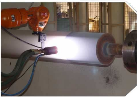
ANTI-WEAR SPRAY ON PAPER INDUSTRY PARTS
