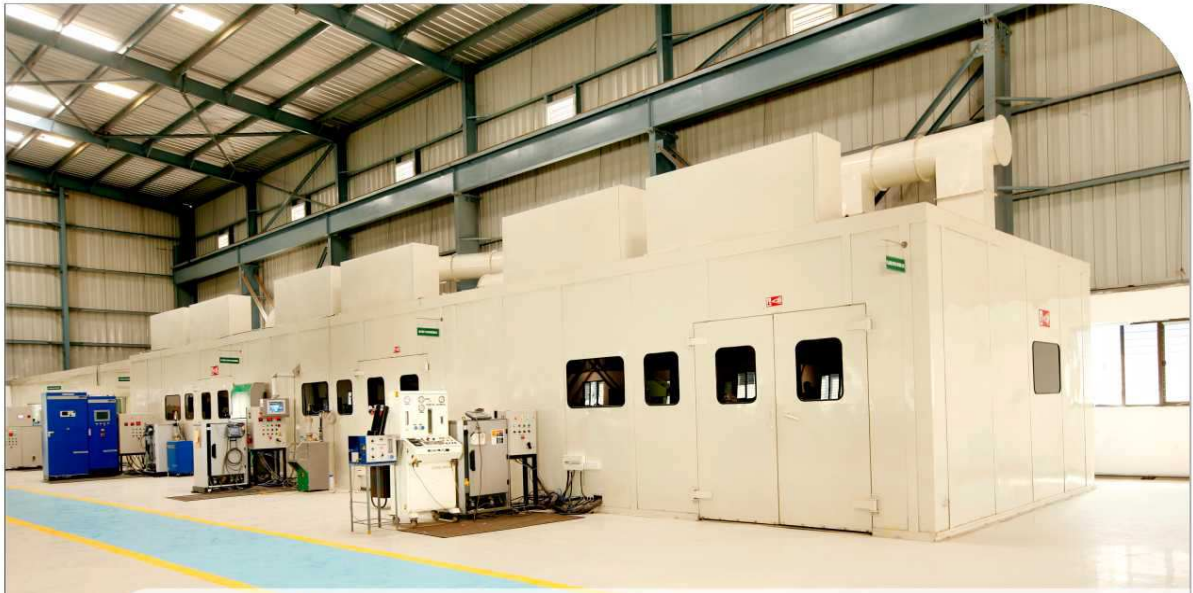
5 ROOMS SETUP FOR DETONATION GUN, HVOF & PLASMA
