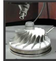
8 AXES ROBOTIC SHOT PEENING MACHINE
